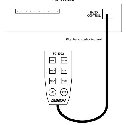
Note: Cable may be extended with ED1753 Hand Control Cable Extension Kit. See PARTS and ACCESSORIES Section.
